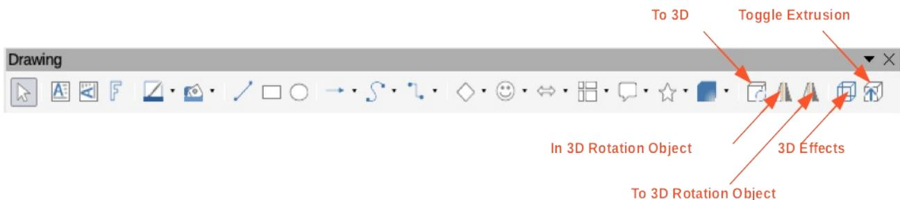
Figure 179: Drawing toolbar with 3D tools
